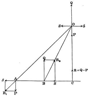
Let  $R_1$  be the resultant of P and S acting at A, and  $R_2$  the resultant of Q and S acting at B. Let the lines of action of  $R_1$  and  $R_2$  meet in O, and let the points of application of these forces be transferred to O. Let  $R_1$ ,  $R_2$  acting at O be resolved [Art. 27 (2)] into forces equal and parallel to their original components.
